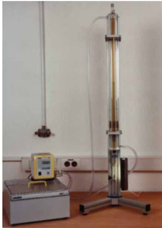
A powder sedimentometer used for determining particle size distributions in fine powders.
