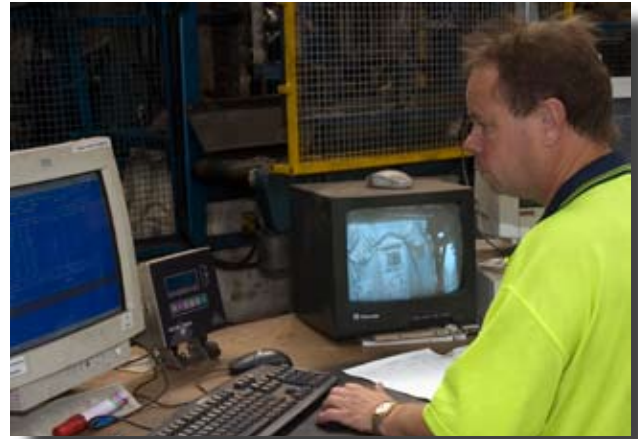
A Storeman uses a video camera to read a bale number and record a bale weight.
