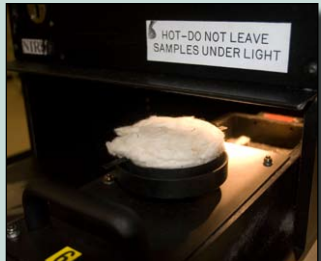
Measuring the ash content of a slice of scoured wool using NIR.
