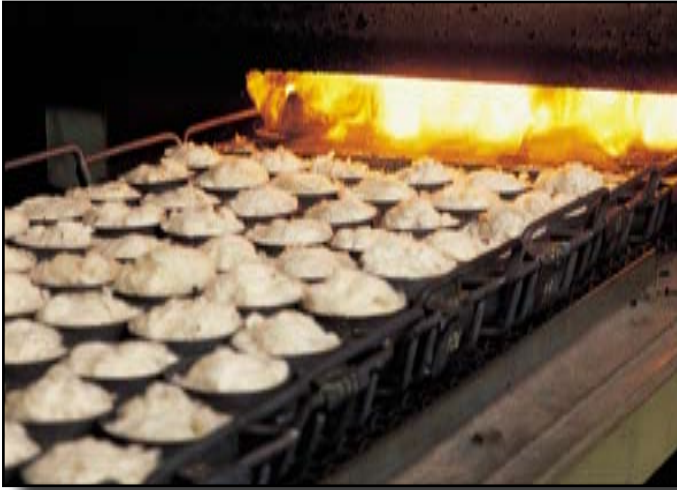
Ashing furnaces burning wool samples at 800°C
