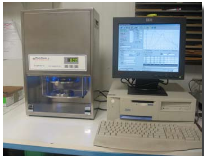
A PhabrOmeter, an instrument designed to quantify fabric properties such as softness.
