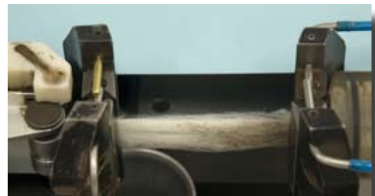
An ATLAS machine grips a staple ready for strength measurement.
