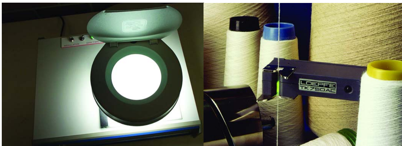
The CSIRO Dark Fibre Detector (left) uses balanced illumination from above and below a thinly spread sample constrained between two glass plates to make objectionable fibres more visible. The SiroCLEAR™ technology (right) is an on-line optical sensing device that detects and removes contamination from undyed yarns.
