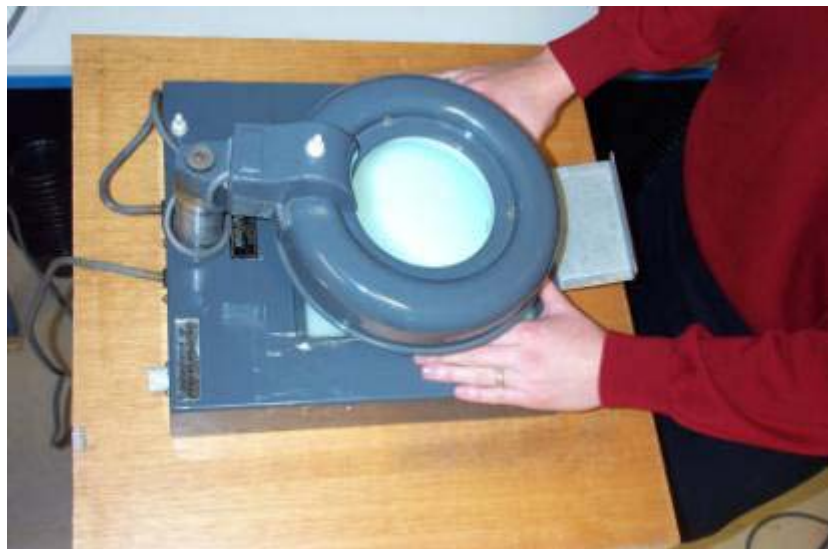
Plate 1: Detection and classification. Prototype CSIRO Dark Fibre Detector used by AWTA Ltd.
