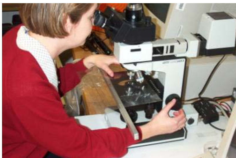
Plate 2: Verification. Microscopic examination of Dark Fibres extracted from the samples. Note the metal bar added to the microscope stage to accommodate an A4 transparency capable of holding up to 25 extracted fibres.
